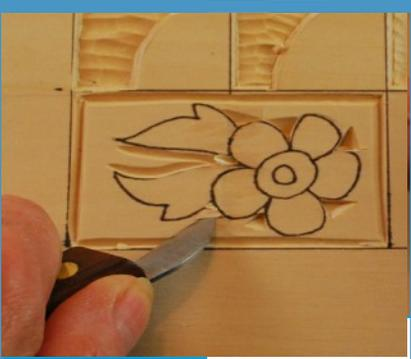
Sharp corners in your patterns can be lifted by using a three stroke cut called a chip carving cut. After the stop cut has been worked around each element of the pattern lay your knife at a low angle along the diagonal of the corner. Make a slice across the diagonal to lift a small triangular chip.
